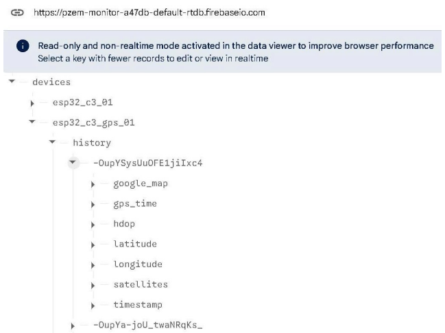
Fig. 8. Sequential data logged in the Firebase history branch.
